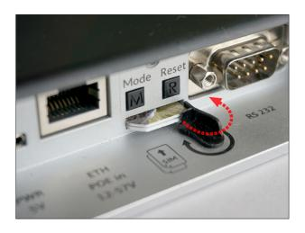
Rotate SIM card lock into position as indicated on above photo to lock both SIM cards.
